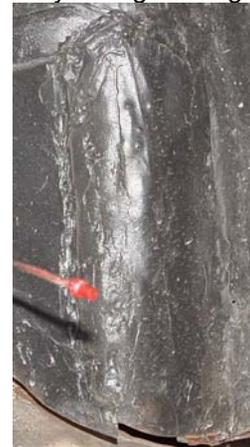
On the outside, it's required to roll the fender lips with the above recommended wheel size. This requires you cut the wheelhouse where it attaches to the fender lip, create a slit every 5 inches or so. Using a hammer and dolly, you fold the lips up to meet the inside of wheelhouse and tack weld them back to the wheelhouse. This is a structural part of the car so it's very important to weld them back.
