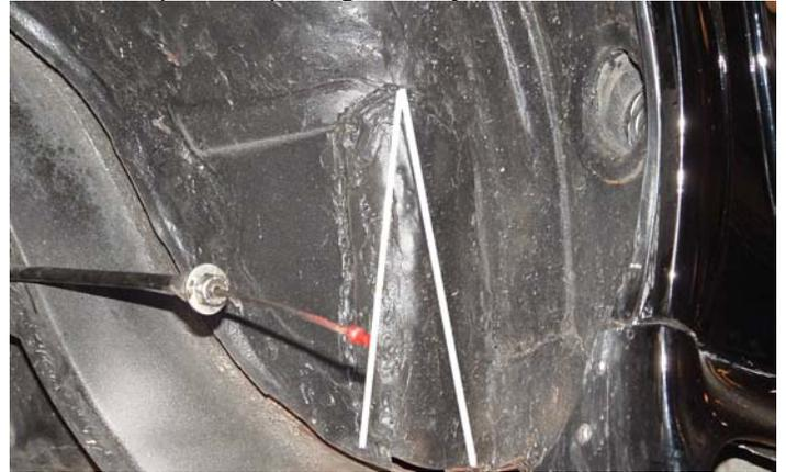
Cut piece of sheet metal to fill the gap, seam weld it in place and undercoat. Repeat the steps on the other side and you're good to go.
