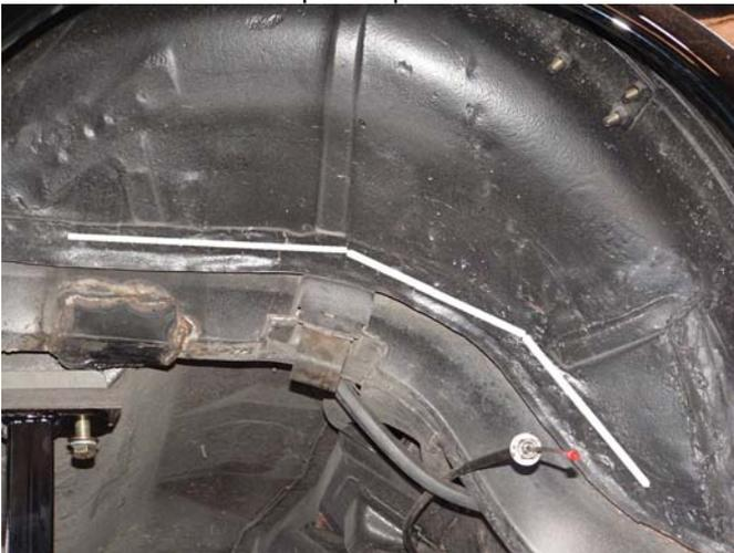
After you align the wheelhouse with the leaf spring, it creates a pie cut opening where you made the initial slit.
