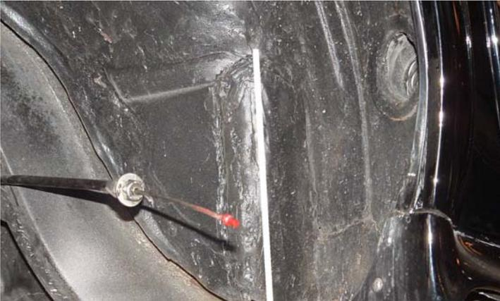
From here, you place a piece of flat stock steel ex. 2x8" usually 1/4" thick, against the wheelhouse where it meets the floor. You're using this as a dolly so you don't create hammer marks in the metal. It needs less movement in the rear, and more toward the front of the car. We used a straight edge and vertically aligned the wheelhouse with the leaf spring. We gained about 1 1/4" in the front section without affecting the inner quarter panel fitment.
