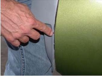
**#1** Start out by matching the end cap up to the car. Find the high point areas, mark with a fine point marker. It's best to go little by little until the end cap begins sitting flush against the car.
