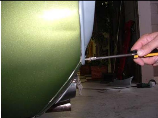
**#6** A sheet metal screw is used to pull in the bottom of the end cap for the finishing touch.
