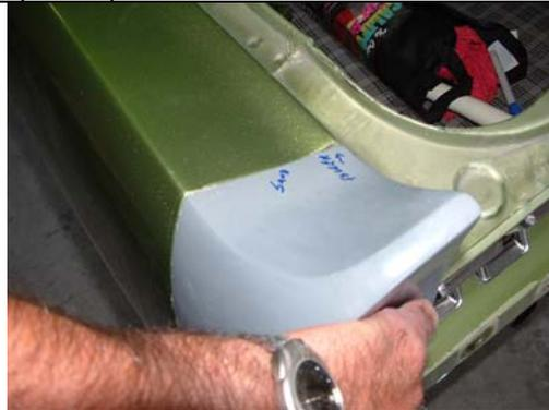
**#4** On the top edge, it should be expected that there may be some minor filler and sanding for a perfect fit. Filler can be minimized by using sheet metal screws into the quarter panel, then flexing the cap down to flex to top edge line into position. This same technique can be used along the side of the end cap.
