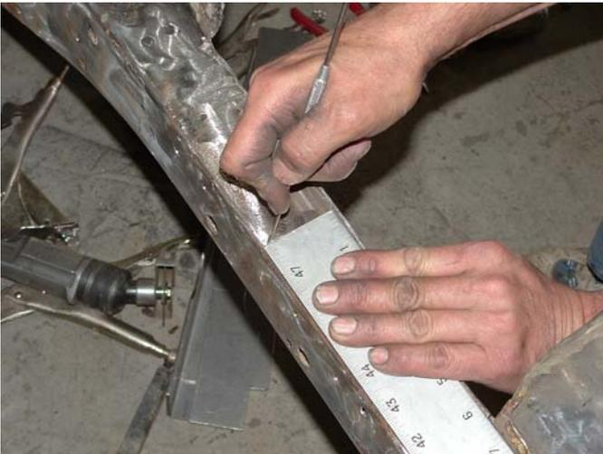
The measurements are provided in the instruction to find the spindle centerline, as well as the template for notching the frame for the spring.
