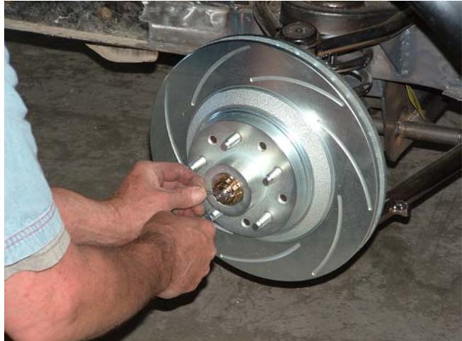
Mount the rotor, snug the nut, install the cotter pin and dust cover to complete the installation.
