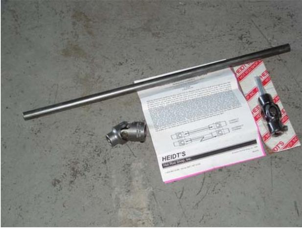
In the Heidt's steering connector kit, you need to specify aftermarket or stock column to get the correct U Joints. There is plenty of rod for the various installations.
