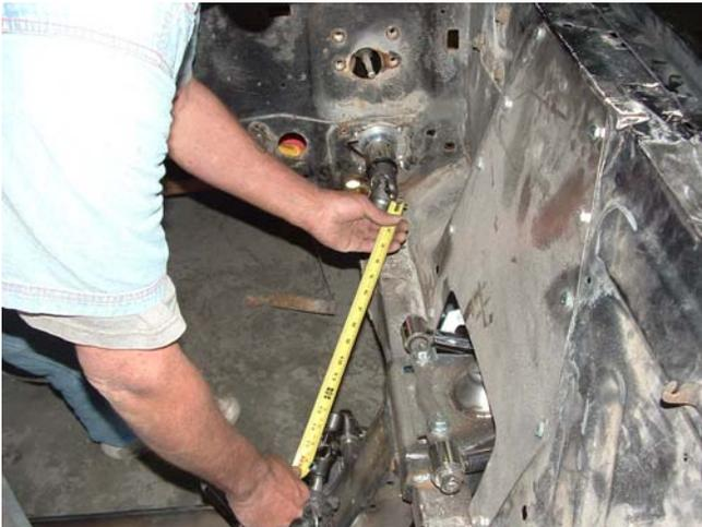
Mount the U Joints to both the column and the steering rack and measure the length of rod you need. Cut to length, install, drill and tap for the set-screw. The Heidt's fender apron cover kit cleans-up the install for a nice finished look.
