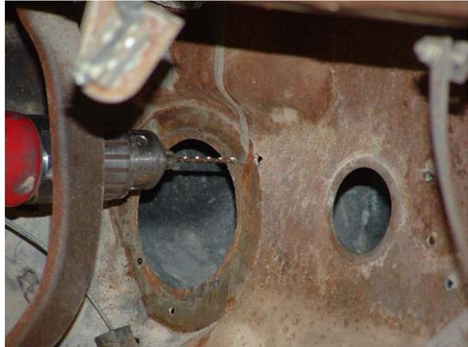
Line up the firewall mount, center punch the holes and drill out the holes. A pilot hole works nice then a 1/4" for finishing.
