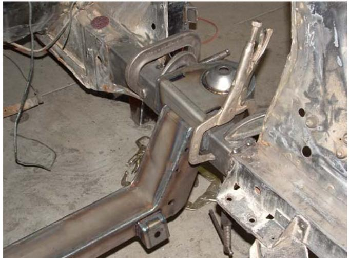
The crossmember is positioned using a jack and tacked into place.
