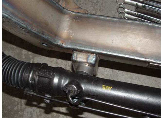
Install the Rack and Pinion with the hardware provided.
