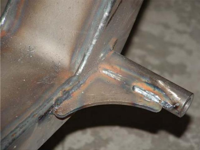
Weld in the lower control arm spacer and gusset. With the more modern, stronger double wishbone system, you do not need strut rods any longer.
