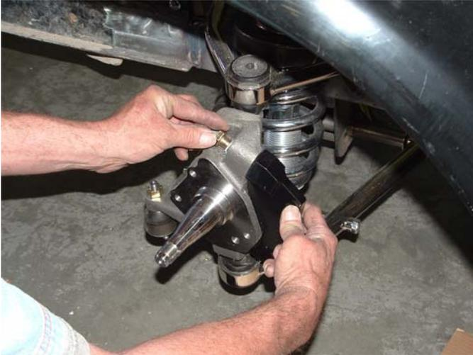
Install the caliper bracket as shown.
