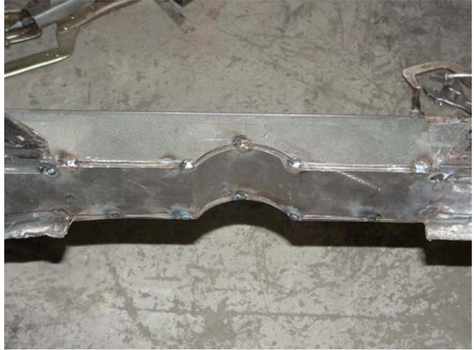
After the notching is completed, the reinforcement plates, provided in the kit, are tack welded into place.
