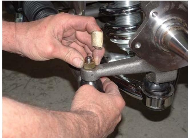
Connect the tie rod ends to the spindle, install the castle nut and cotter pin.
