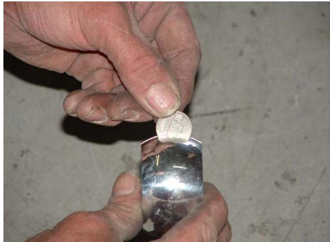
Use a nickel or similar object to spread out the ball to slide onto the column. It works best to install the bottom half of the firewall mount, rest the ball on the lower half, then install the upper half. It's important to loosely tighten all hardware until everything is in place to avoid stripping the aluminum threads. A good thread locker is also in order. We used 1/4 "x20 x 1 1/4" stainless socket head allens to finish off this part of the install.
