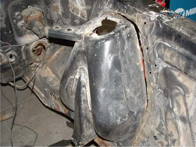
The conversion is started by removing the shock towers. A plasma cutter works the best here, but a cutting torch or saw works almost as well. Remove the lower control arm mounts as well to make room for the large crossmember supplied in the Heidt's kit.
