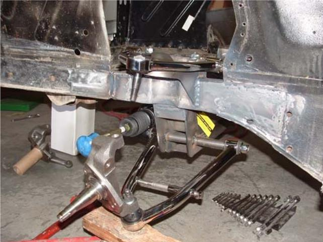
Next install the lower control arms, the upper control arms and the standard 2" drop spindle to retain stock ride height. We selected the tubular lower control arms for extra stability and a show car finish.
