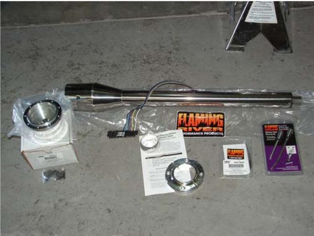
We chose the Flaming River Industries, GM splined, polished stainless 30" tilt column for our 65 Mustang. Also note the 2" ball and socket firewall mount and polished aluminum 9 bolt steering wheel adaptor for a super sanitary finished look.
