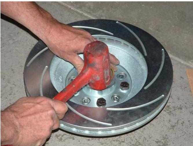
Install the bearings and seal to the rotor. Make sure to grease the bearings and races prior to installation.
